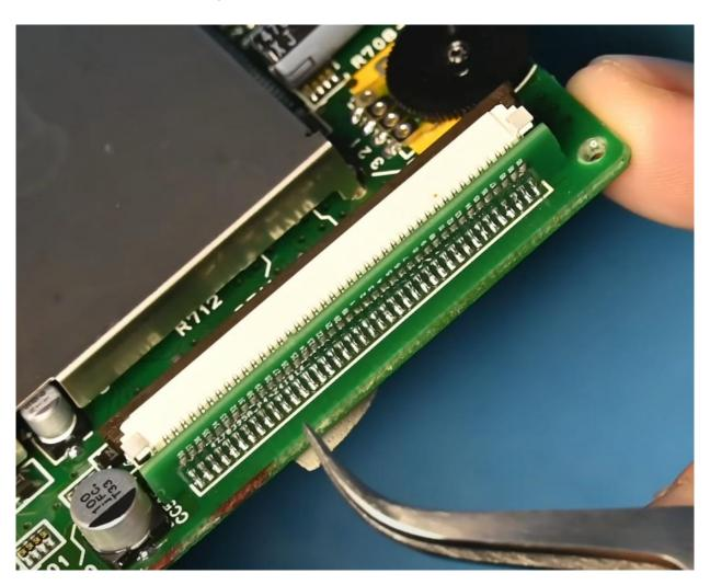
Connect the FFC ribbon to the main board and HuCard connector board as shown.
