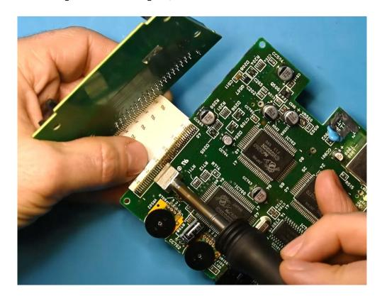
Apply fresh solder to the HuCard connector pins, then using a desoldering gun or solder sucker, desolder the connector from the factory HuCard connector board.
