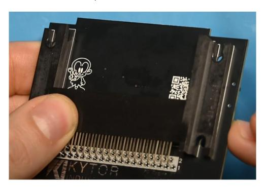
Apply solder to the large grounding pad.
