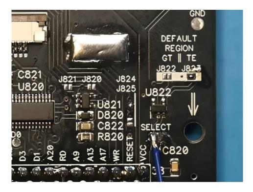
Solder the reverser rider to the pads where the factory ribbon was removed. The FFC connector should face towards the metal shielding. Angle the FFC connector parallel to the main board or slightly upwards.
