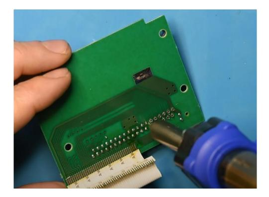
Carefully line up the HuCard connector footprint with the printed footprint layout, and solder all pins into place on the reverse side.
