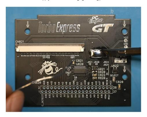
[RF mod only:] Close jumper J823 to set the default boot region to TE <u>or</u> close J822 to set the default boot region to GT. Solder one end of the provided wire to the SELECT pad.
