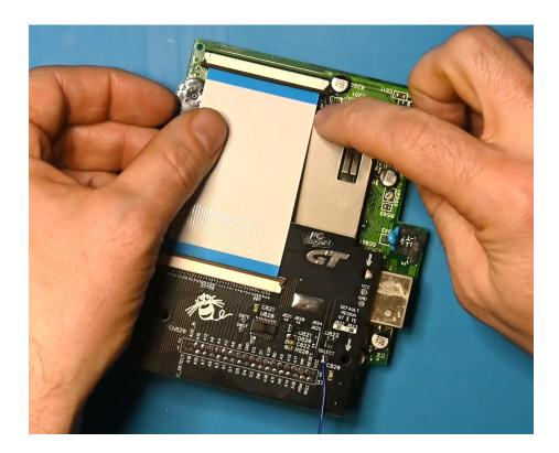
Solder the other end of the SELECT wire to the pad on the control board shown and reassemble in reverse order.
